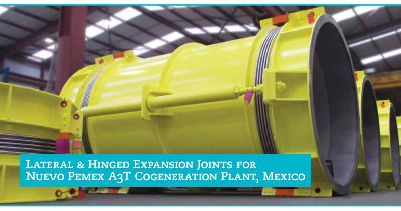
MACOGA has completed the production of 4 Lateral Tied DN2300 MWL units and 4 Hinged DN2300 for the Nuevo Pemex cogeneration plant in Tabasco.
