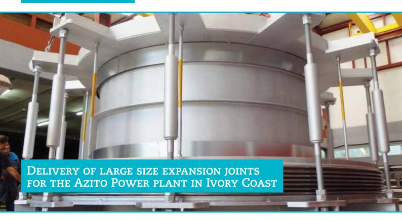
An In-Line Pressure Balanced MPB-I DN 4000, 14 units Gimbal DN 2200 and 7 units Hinged DN 2200 have been shipped from MACOGA for the Azito Power Plant expansion in Ivory Coast.
